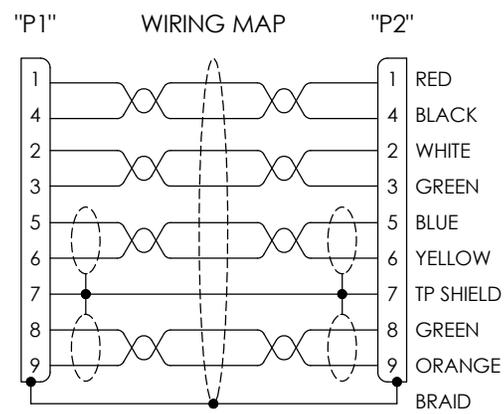
UL STYLE 20276, USB3.0 HIGH FLEX CABLE, (2) TWISTED PAIR, 28AWG WITH ALUM/POLY, DRAIN WIRE AND SPIRAL SHIELD, (1) UNSHIELDED TWISTED PAIR, 26AWG, (1) UNSHIELDED TWISTED PAIR, 22AWG, OVERALL ALUM/POLY AND BRAIDED SHIELD, JACKET: PVC, BLACK (NOM DIA. .276" [7.0]; FLAME RATING: UL VW-1; MIN. FIXED BEND RADIUS: 5X O.D.; MIN. MOVING BEND RADIUS: 10X O.D. )
