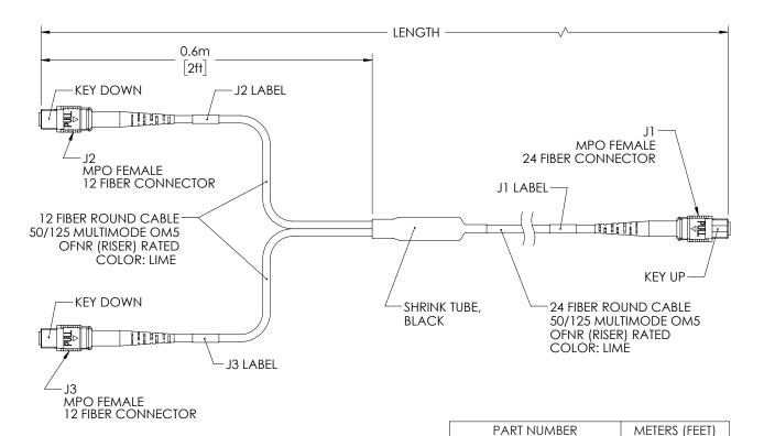
UNLESS OTHERWISE SPECIFIED LEADING DIMENSIONS ARE INCHES DIMENSIONS IN [] ARE MILLIMETERS TOLERANCES: .X=± .2 [5.08] **FRACTIONS**
