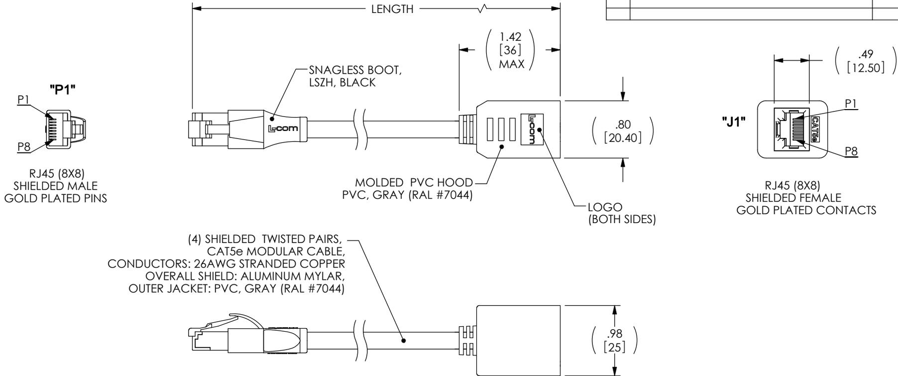
(4) SHIELDED TWISTED PAIRS, CAT5e MODULAR CABLE, CONDUCTORS: 26AWG STRANDED COPPER, OVERALL SHIELD: ALUMINUM MYLAR, OUTER JACKET: PVC, GRAY (RAL #7044)
