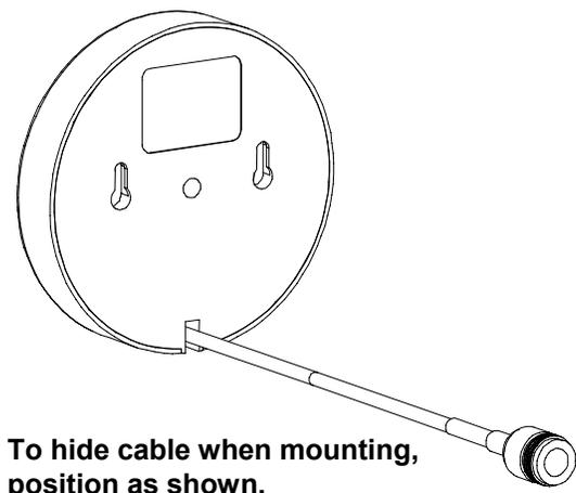
To hide cable when mounting, position as shown.
